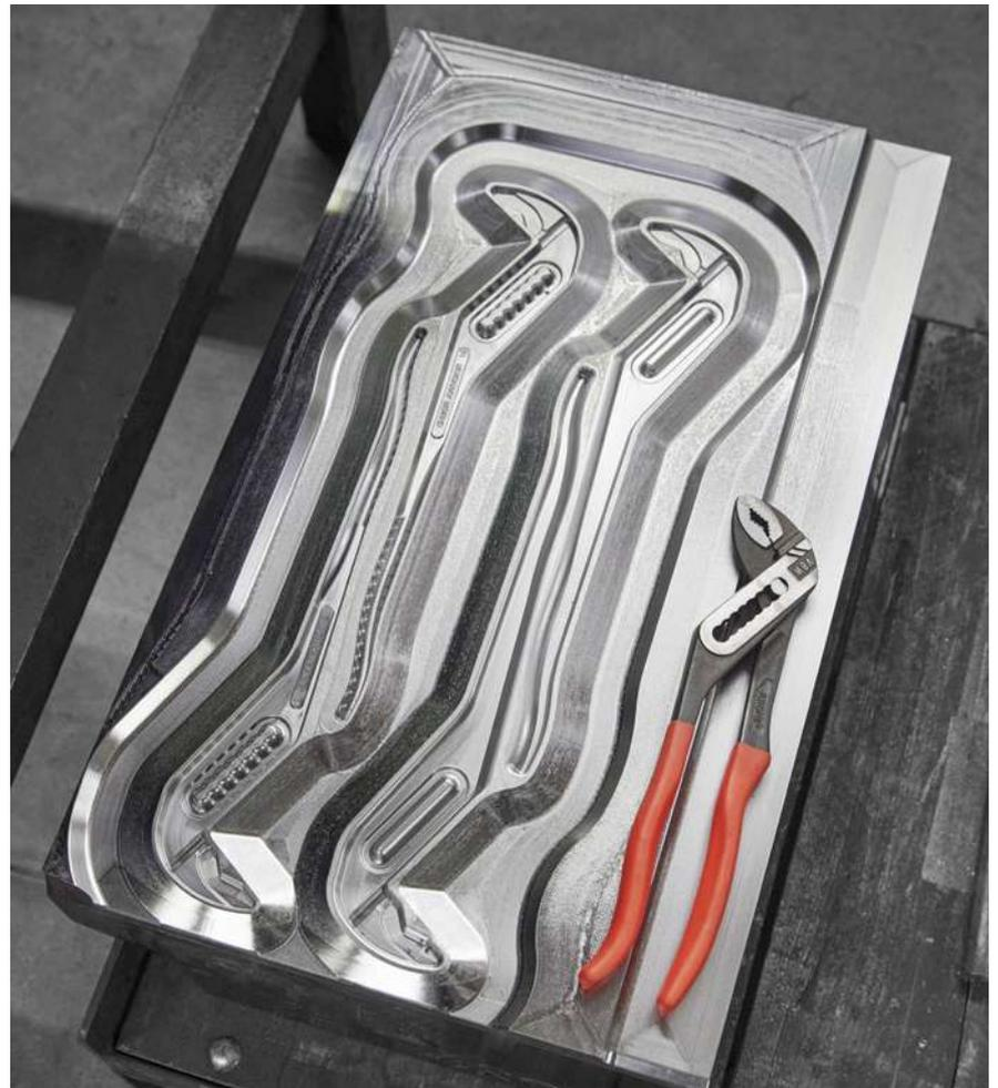
**Enhanced grip:** The STAHLWILLE die forge manufactures forged parts using the Starrag Heckert H55 machining centre.
