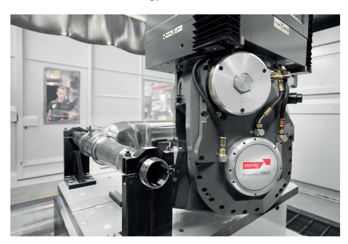
A prime example of high-tech: One Russian customer was able to rough and finish landing gear housing for aircraft in one clamping operation using a Droop+Rein portal-type milling machine from Bielefeld.
